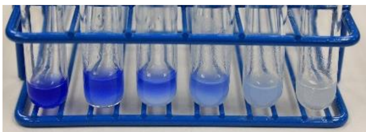
Figure 3. Ammonia test results over the course of the copper precipitation reaction.
