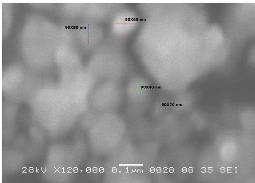
**Figure 1** A) Scanning electron micrograph of AgO nanoparticles with their respective shapes and size and B) energy dispersive spectroscopy systems map spectrum confirming the presence of silver in the stock solution.
