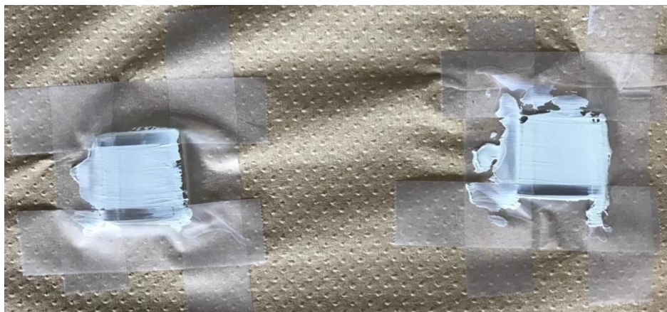
Figure 2. Titanium dioxide semiconductor paste applied to the tin(IV) oxide transparent conducting oxide-coated substrates.
