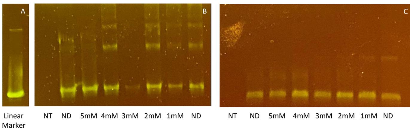
**Figure 4:** A) Linear marker; B) TopoisomeraseII $\alpha$  assay with Ethyl 8-methoxycoumarin-3-carboxylate; C) TopoisomeraseII $\alpha$  assay with 3-acetyl-8-methoxychromen-2-one, NT – no topoisomeraseII $\alpha$  added (negative control), ND – no coumarin added (positive control), rest of the lanes indicate the concentration of the coumarin product added to each reaction tube to inhibit the topoisomeraseII $\alpha$  enzyme.
