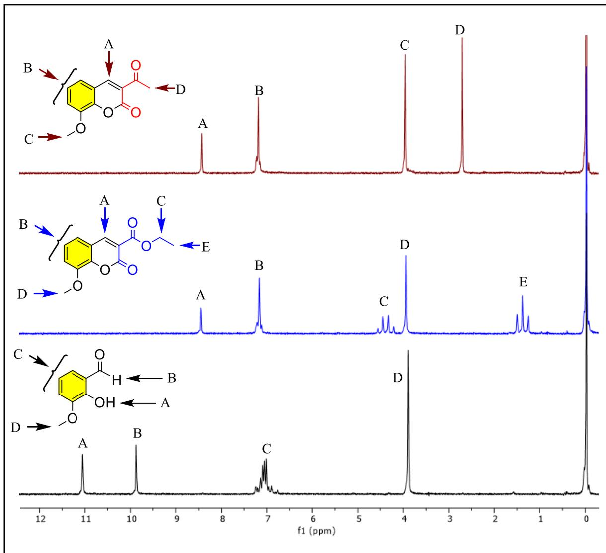
**Figure 2:** Stacked <sup>1</sup>H NMR spectra showing successful conversion of *o*-vanillin (bottom spectrum) to ethyl 8-methoxycoumarin-3-carboxylate **1** (middle spectrum) and 3-acetyl-8-methoxychromen-2-one **2** (top spectrum).
