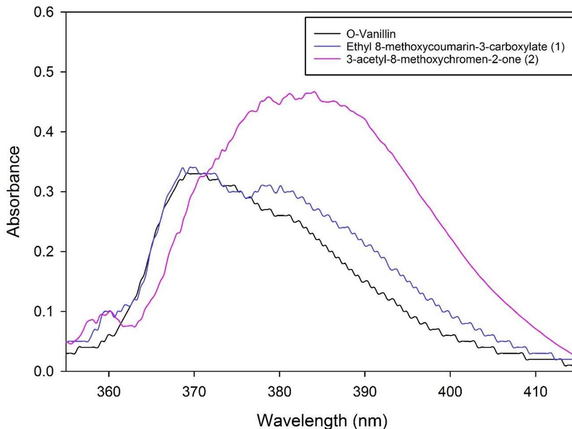
**Figure 3:** Comparison of the UV-Vis spectra of starting material (o-vanillin) and the two synthesized coumarins. The spectra show a bathochromic shift in the absorbance peaks when the product is formed.
