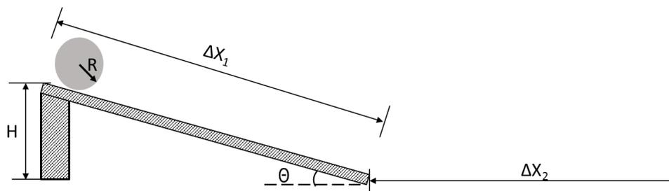
**FIGURE 1.** Schematics of the Scenario - Rolling object on the inclined plane.  $\Delta X_1$ : Displacement on the ramp,  $\Delta X_2$ : Displacement on the floor,  $\theta$ : Angle of the ramp,  $H$ : Height of the ramp,  $R$ : Radius of the rolling object
