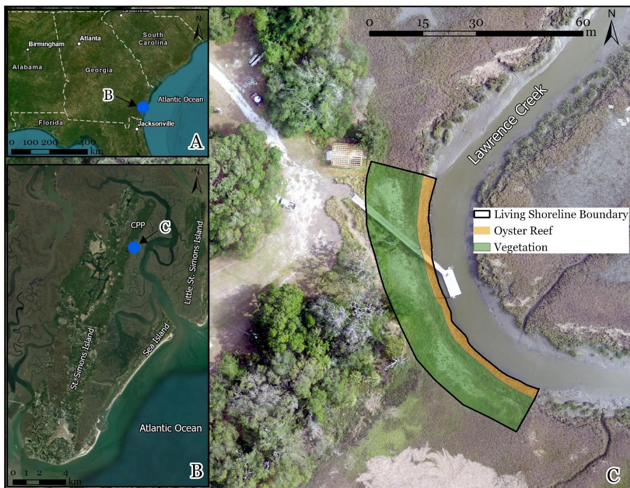
Figure 1. Location of the living shoreline (A) on the Georgia coast, (B) at Cannon's Point Preserve (CPP), St. Simons Island, and (C) on the west bank of Lawrence Creek, where shaded polygons show the areal extent of the restored oyster reef and vegetated salt marsh. Maps A-B were created using ArcGIS® software by Esri. ArcGIS® and ArcMap™ are the intellectual property of Esri and are used herein under license. The image of the living shoreline site (C) was provided by Georgia Department of Natural Resources.
