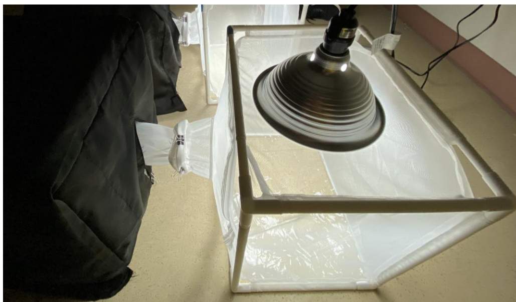
Figure 1. Our phototaxis experiment setup. The covered cage on the left is occupied with Eristalis tenax (starting cage) and the empty cage with experimental lighting on the right is the receiving cage. The two cages are connected via sleeve openings that are clipped together. The pictured experimental environment is white LED light.
