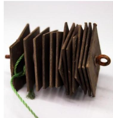
**Figure 1.** Hester Dendy sampling device.
